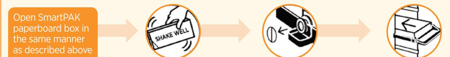
Open SmartPAK paperboard box in the same manner as described above for the Coca-Cola Freestyle 8000 and 9000 dispensers. Vigorously shake each cartridge for 10 seconds (leave inner seal on the cartridge while shaking). Insert paperboard cartridge into black plastic tray, remove inner seal; align cartridge with the tray. Insert cartridge and plastic tray into appropriate slot.
