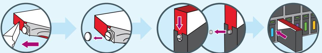
Open SmartPAK paperboard box by removing perforated corner. Pull off white dust cap. Insert paperboard cartridge into black plastic tray and remove inner seal. Insert cartridge and plastic tray into appropriate slot.\*
