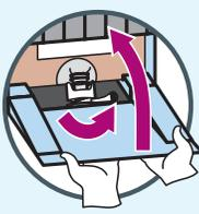
Position NNS bag-in-box with arrows pointing down and white lever secure (lever moves left to right to close; right to left to open).
