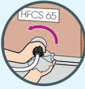
When disconnecting bag-in-box, place clean cloth under connector to catch any sweetener drips. Rinse connector in a cup of warm water prior to connecting a new bag-in-box.
